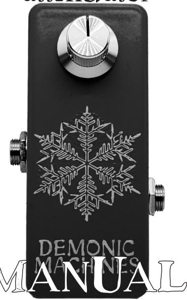
STEP 1: Connect the Amp Chiller to your amp's effects loop. IMPORT-ANT: Make sure to place the Amp Chiller in the effects loop and not between your amp and your speaker.
