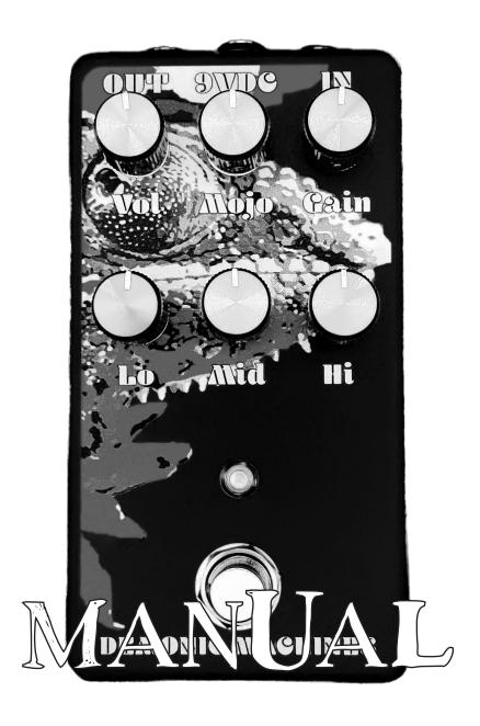
The CHAMELEON OD is an extraordinary soft-clipping overdrive circuit designed to provide a wide range of tonal options. It incorporates internal DIP switches that offer over 4,000 variations for clipping flavors. Additionally, it features an active 3-band EQ capable of delivering up to 10dB of boost or cut.
